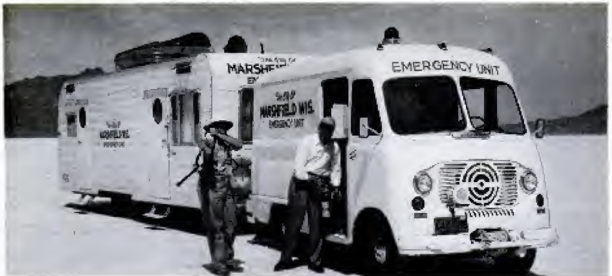
Disaster unit carries portable power unit and winch, axes, ladders, stretchers and aluminum boat on roof
